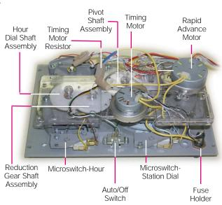
• *Check the clock motor (or timing motor).* The clock motor must operate continuously whether the controller is on or off, in order to keep proper time; therefore, this motor may fail after an extended time. Verify that the motor is receiving proper voltage. Then set the hour to the correct time and wait one hour. If the hour dial has not moved, replace the motor.
