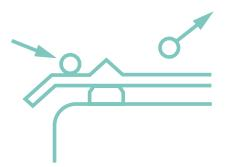
3. Set each switch bracket so the four pins remaining barely touch the surface of the switch breaker arm before coming into contact with the ramp.
