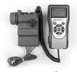
Connect the transmitter's infra-red cord to the controller's socket
